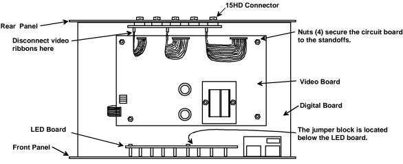
Overhead view of video board on top of digital board.
